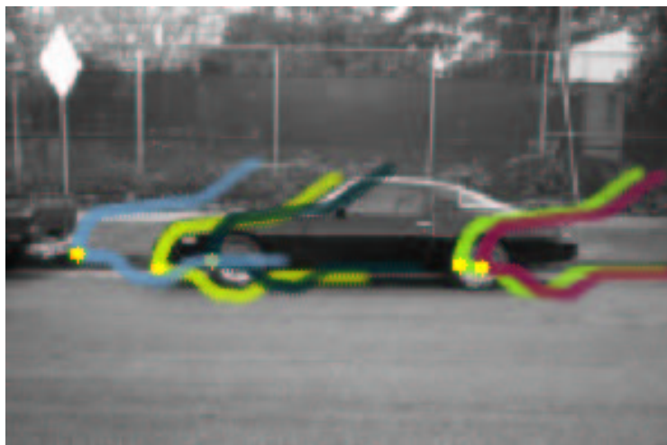
Figure 4: Landmark candidates are extracted by matching local edge information to the generative model and choosing the best K candidates for each landmark. Here we show the best 5 candidates matched to the edge feature of the front bumper. For each candidate, we extract a square ( 21 \times 21 ) patch. Using a PCA codebook computed from a large set of positive and negative training examples, we then extract the first 10 principal components from the patch. These values are appended to create the feature vector for the image.
